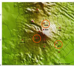
Figure 2: Map of monitoring stations at Popocatepetl volcano. NOVAC instruments have been installed at Tlamacas (PPM), Colibri (PPC) and Chipiquixtle (PPX) stations (source: Alicia Martínez).
